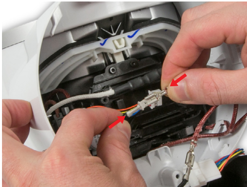
71 Connect the black heater wires.
