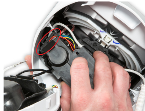
75 Carefully locate the ledge on the cover into the gap in the terminal plate. Important: it is crucial that there are no wires trapped between the cover and the plate.
